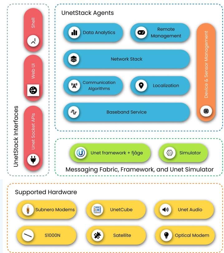
The UnetStack ecosystem is built around the following three core pillars which together provide a complete foundation for developing, simulating, and deploying underwater and hybrid communication networks.
