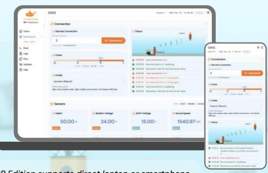
SWIS – ADCP Edition supports direct laptop or smartphone access with an intuitive UI, as well as integration with cloud servers, FTP servers, and data loggers for automated data collection.
