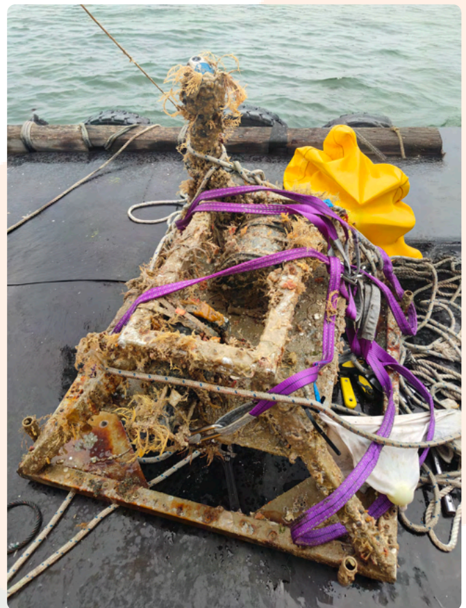
The lander on recovery, showing the extent of biofouling after four months in the water.
